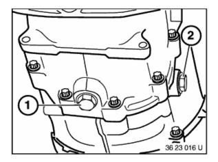
Unfasten drain plug (1) and filler screw (2). Clean drain plug and screw in. Tightening torque, refer to Technical Data 23 00 4AZ Top up transmission fluid until it overflows. Tighten in filler screw (2). Tightening torque, refer to Technical Data 23 00 4AZ
